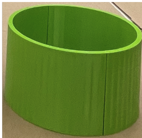
Figure 55. Extended nosecone mold (Height 10 cm)
